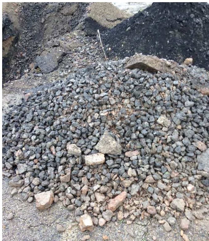
Photograph No. 8 – Excavated Brick and Concrete Debris with Black Gravel Fill from LT-5
