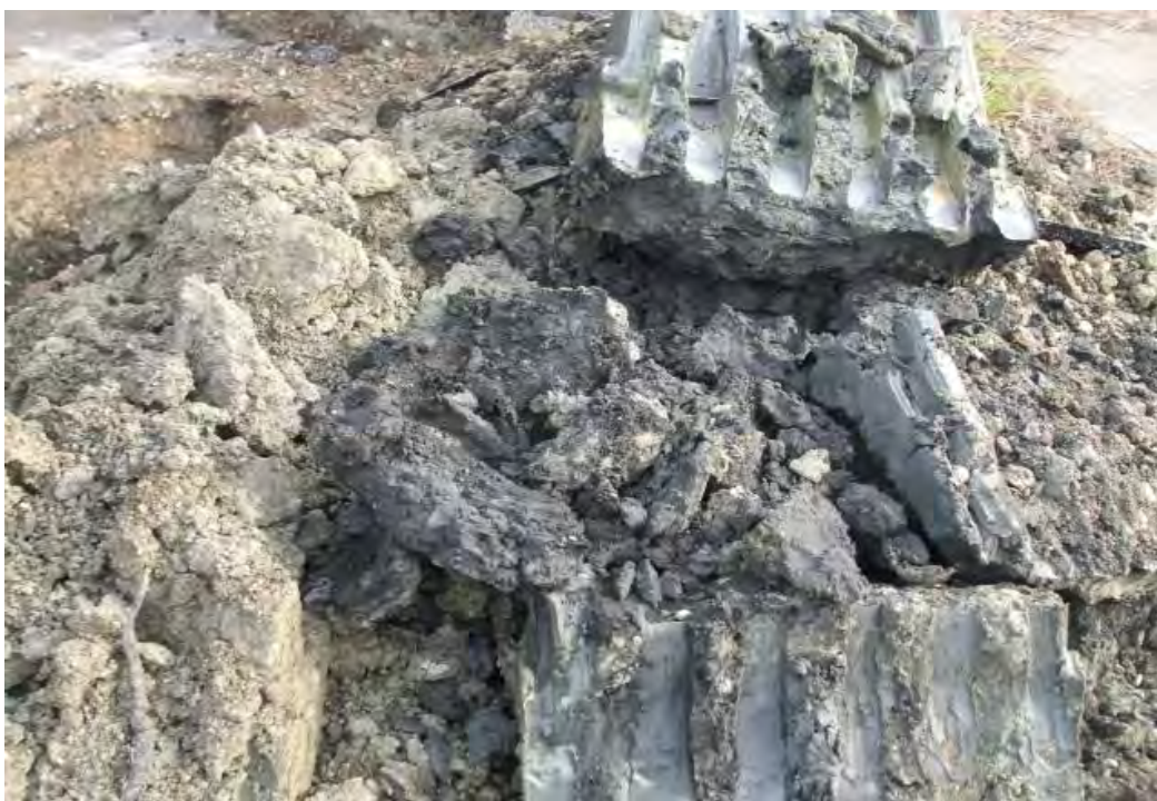
Photograph No. 20 Excavated Brown Silty Clay Fill and Underlying Black to Bluish Gray Organic Silty Clay Fill from TP-12
