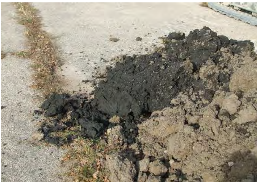
Photograph No. 16 Excavated Brown Silty Clay Fill and Black Organic Silty Clay Fill Soils from TP-10
